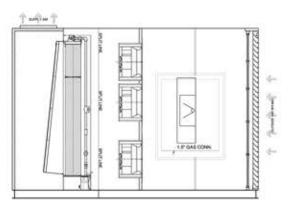
The Make-Up Air Units are designed with both heated and cooled systems, to improve the quality of the air that is exhausted by other mechanical means. This units pulls in the fresh, tempered air from outside your building to replace and improve existing air that cannot be recirculated within the building.
