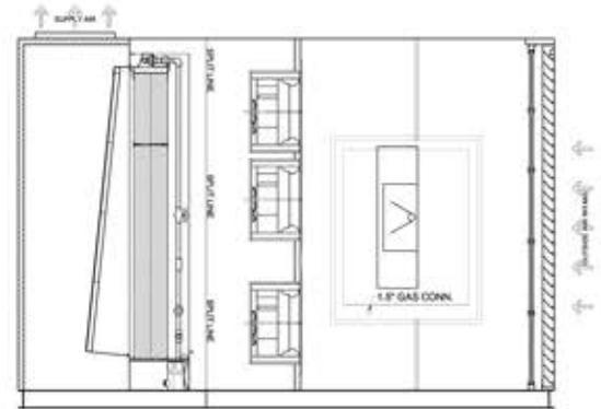
The Make-Up Air Units are designed with both heated and cooled systems, to improve the quality of the air that is exhausted by other mechanical means. This units pulls in the fresh, tempered air from outside your building to replace and improve existing air that cannot be recirculated within the building.
